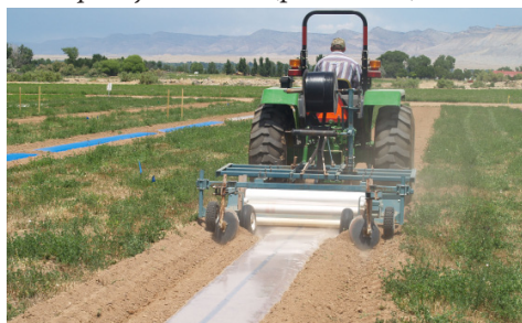
A weed mulcher is being used to lay plastic mulch for soil solarization.
